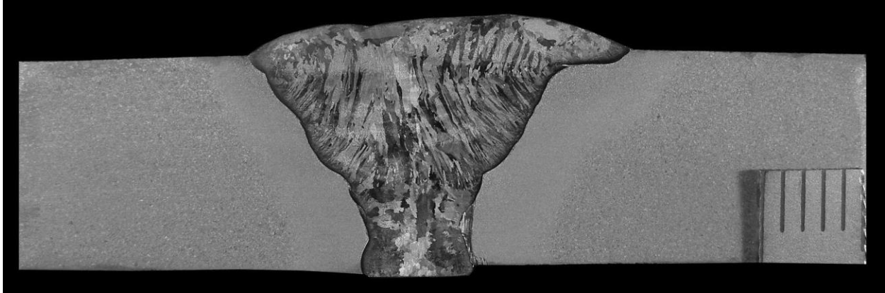
Figure 9. Thor™ 115 welded with S Ni 6082 filler metal; etchant: Nital; magnification 2x; quality level: B.
